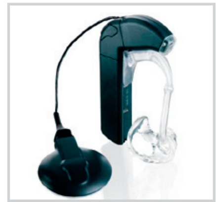
Figure 2. The externally-worn speech processor of an EAS implant (Photo courtesy of MED-EL)
